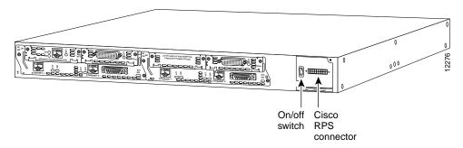
Step 3 Connect the DC-input end of the cable to a Cisco RPS rear-panel connector as shown in Figure 14 or Figure 15.
